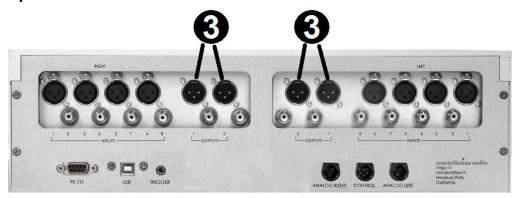
The inner six XLR connections on the rear of the Virgo III are outputs. The signal at these outputs is the same—it does not matter if you use output 1 or output 2. To remove an XLR plug, push on the tab on the connector body and pull the plug out.
