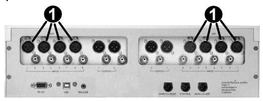
On the rear of the Virgo III preamp there are eight XLR inputs, four on each side. As you are looking at the rear panel, the left four XLR inputs are for the right channel, the right four inputs are for the left channel. Underneath each jack is the corresponding input number. Use of XLR connections is recommended for the best possible audio quality. To remove an XLR plug, push on the tab above the jack and pull the plug out.
