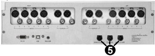
These connect to the power outputs of the Virgo III's power supply. The Virgo III includes special spiral-wrapped, gold-plated copper cables designed for aerospace use. Each cable is rated to handle 30 amps.
