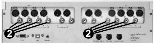
These unbalanced inputs are provided as a convenience for use with unbalanced signal sources. Whenever possible, we recommend using XLR connections instead. Connecting to an unbalanced source is handled in the same way an XLR balanced source.
