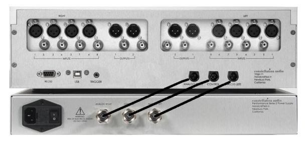
The Virgo III's separate power supply (bottom component in the picture above) must be connected to the Virgo III main chassis (top component in the picture above) as shown above before you plug the unit into a wall. Make sure the power switch on the power supply is in the off (O) position. The supplied cables are spiral-wrapped, gold-plated copper designed for aerospace use, and can handle up to 30 amps. Only these cables should be used between the power supply and the Virgo III.
